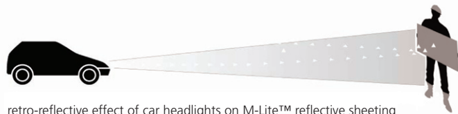
retro-reflective effect of car headlights on M-Lite™ reflective sheeting
