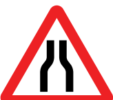
ROAD NARROWS AHEAD P-517A
